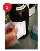
Peel label with RFID sticker off the Hydranal bottle.
